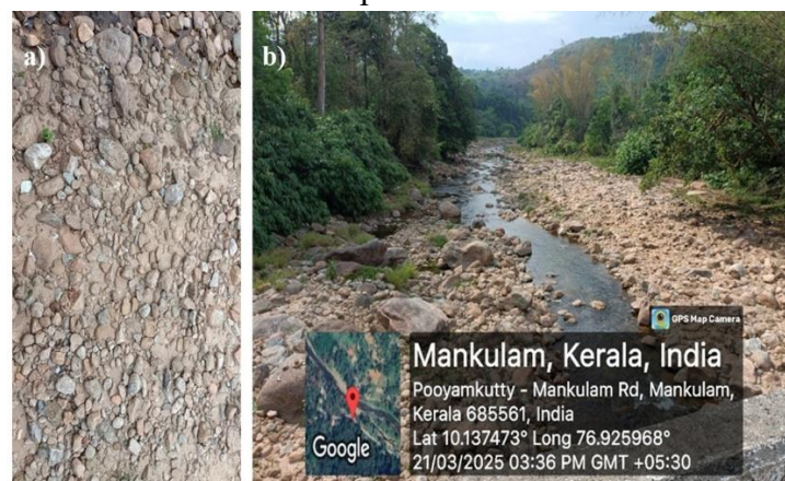
Figure 25 (b): Images taken during field visits verifying the features at River Style 1, showing (a) cobbles and pebbles, and (b) a boulder present in the riverbed
