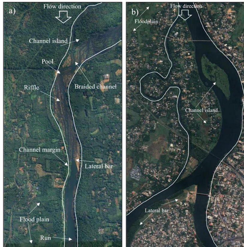
Figure 37 (a) and (b): Google Earth imagerys of River style 10 illustrating the key features of the style such as lateral bars, braided channel, channel island and flood plain.
